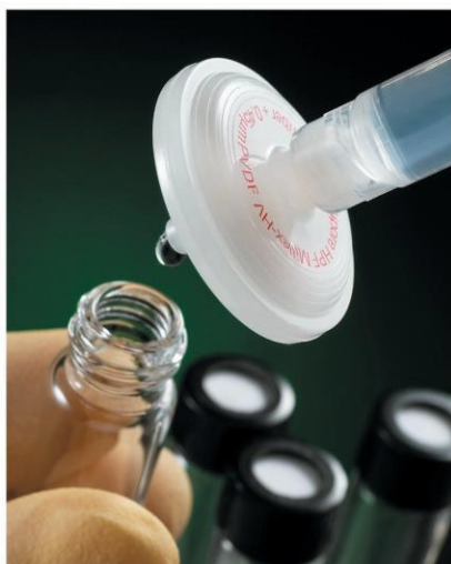
Figure 6-2: Syringe filter for dissolved metal sampling
